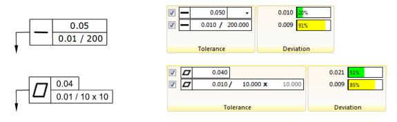
Independent from the way the tolerated element was measured, a Chebychev compensation element is calculated for the straightness and flatness evaluation which results in a standardized evaluation according to ISO 1101.
