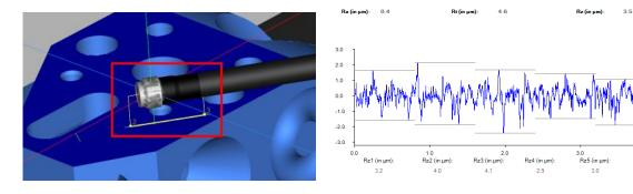
The following roughness parameters are automatically calculated: Ra, Rq, Rz, Rp, Rv, Rt, Rmax
