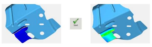
Before measuring the surface, additional areas can be defined on the CAD model. Points that lie outside the defined areas are not projected onto the CAD surfaces. This can be used, for example, to leave out clamps of a fixture or to restrict areas of a large CAD surface.
