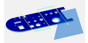
Transfer paths on which the line scanner does not pick up any points are drawn in blue in the distribution.
