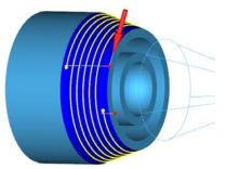
The two new distribution methods "Spiral clockwise" and "Spiral counterclockwise" are available for measuring cones.
